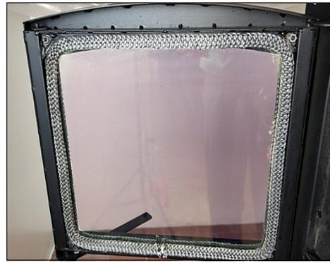
Figure 4 - Door Gasket in Good Condition
