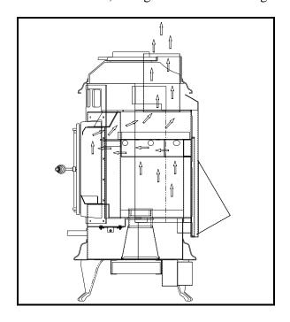
FIGURE 19. EXHAUST AIR FLOW
