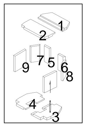
FIGURE 22. PLACEMENT OF VERMICULITE INSULATION
