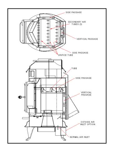
FIGURE 18. SECONDARY AIR FLOW
