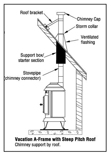
FIGURE 9. VACATION A-FRAME WITH STEEP PITCH ROOF
