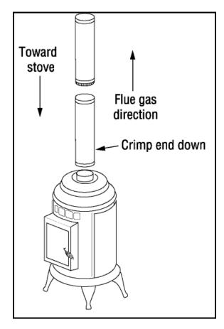
FIGURE 6. CHIMNEY CONNECTOR AND FLUE COLLAR
